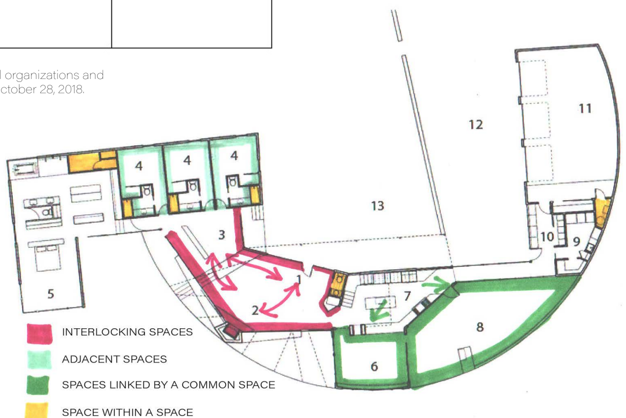
Figure 24 (above): Non-exhaustive diagram of spatial relationship examples in Sage House's design. FROM: Architectural Digest, 2018.
